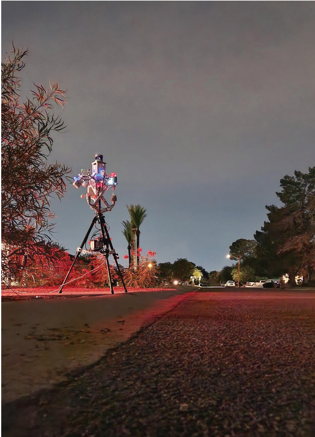
Figure 5. OTTO during acquisition in Phoenix, Arizona, recording the nighttime effects of the overheating surfaces of the city. Image Source: © Vibrant Fields.
