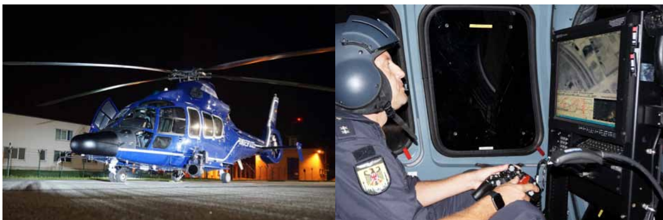
Fig.11 - Left: The Eurocopter 155 with four thermal imaging cameras. Right: The thermal imaging cameras can spot individuals from several kilometers away at night. Chemnitz, Germany. 2015. Photos by M. Unger.
